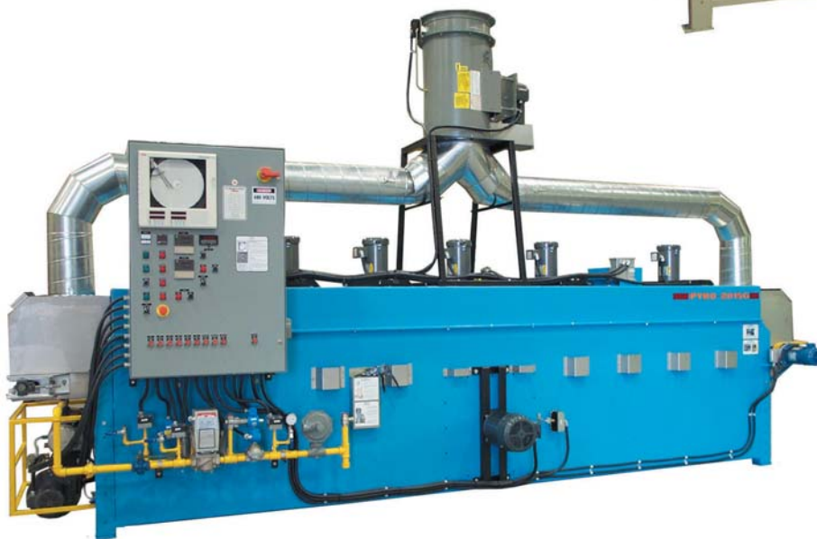
PYRO-2015G Automotive Valve springs stress relieving gas fired (5-7 min. cycle time)
