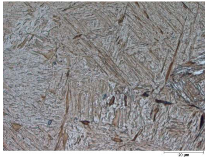
Figure 10- Surface microstructure of S/N 1 as-quenched. 2% nital. (1000X)
