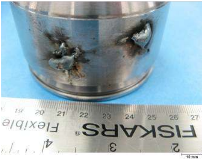
Figure 3- Weld spatter noted on S/N 6. (1X)
