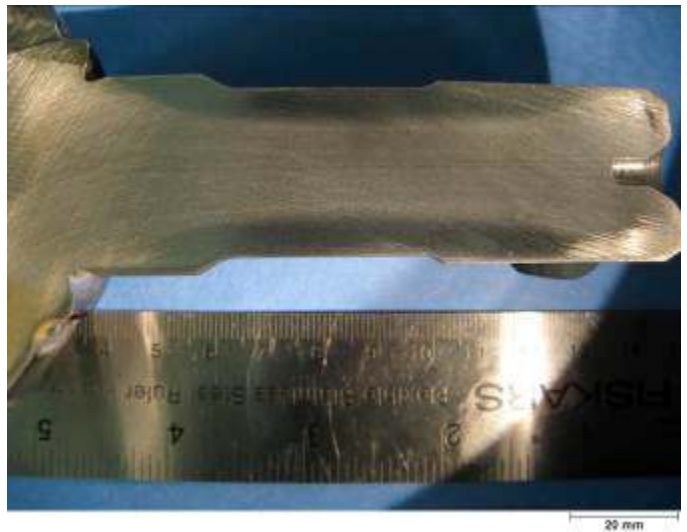
Figure 4- Representative induction pattern noted on all samples. (0.85X)
